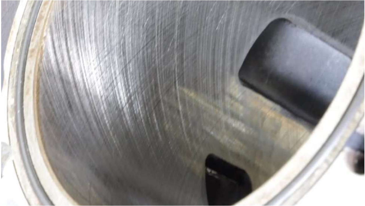
Cylinder-wall roughness (image captured from Brian's presentation)
