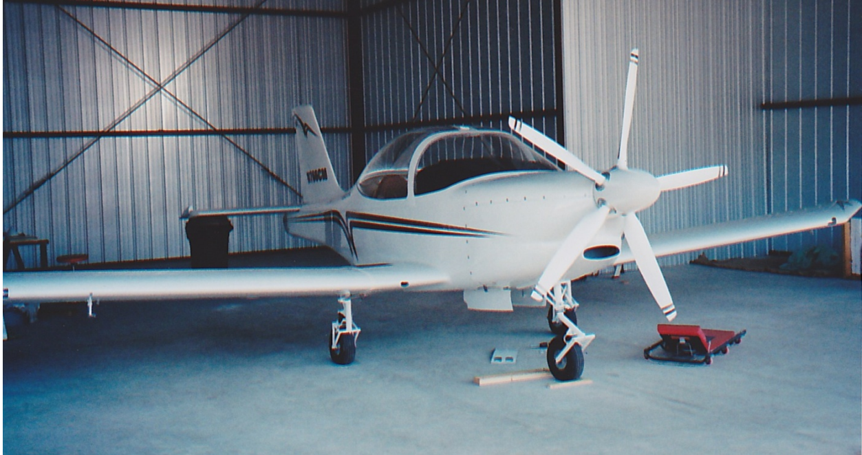
Alfa HB-207 that Conrad built in 2010. Powered by a VW-Porsche 110 hp flat-four engine, it has retractable gear and an adjustable prop. It cruises at 152 mph.
