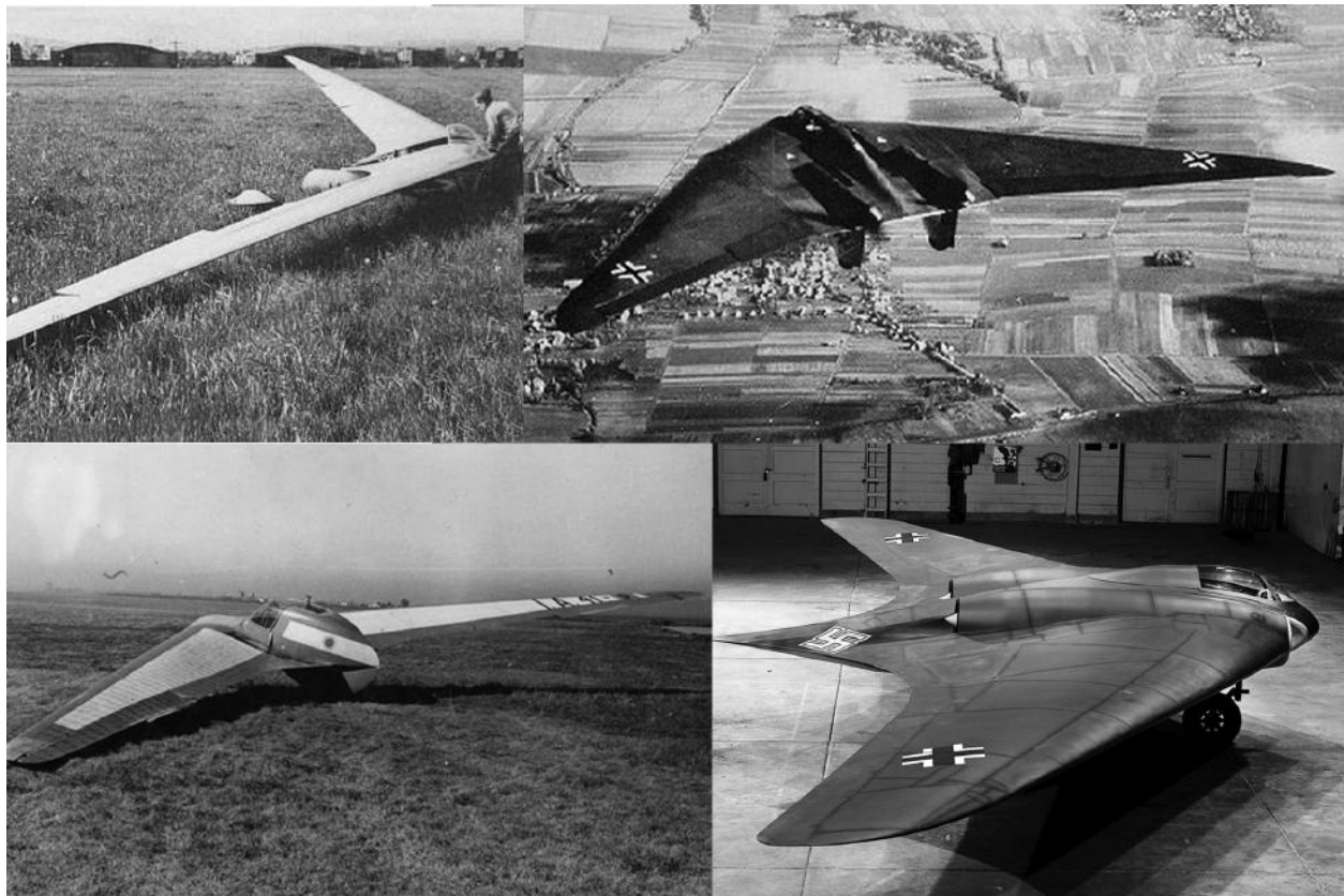
The Horten brothers first tested and proved their tailless flying wing gliders from the slopes of the Wasserkuppe. With WWII they went on to produce very futuristic designs, including flying wing jet fighters.
