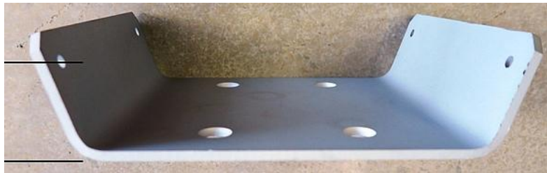
New engine plate is 1/2" shallower than the old one
