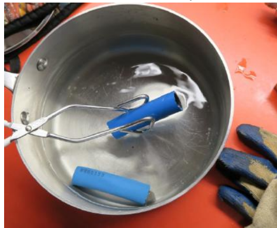
Boiling and softening the hoses
