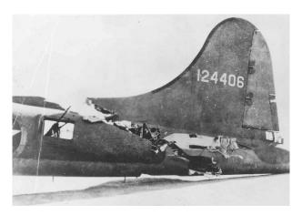
This is a close-up of the damaged tail of Boeing B-17F bomber "All American III". The left horizontal stabilizer was torn completely off, and the aircraft was nearly cut in half in flight after a collision with an Me-109 over Tunis. She was able to land safely at her home base in Biskra, Algeria.
