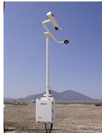
New AWOS-III weather station at Front Royal Airport (KFRR). Not shown is the closet of computer gear in the terminal building.
