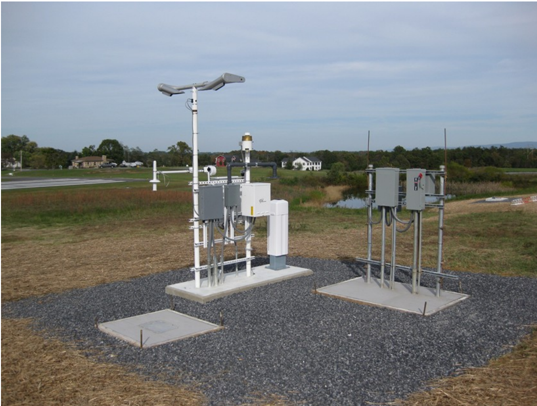
New AWOS-III weather station at Front Royal Airport (KFRR). Not shown is the closet of computer gear in the terminal building.
